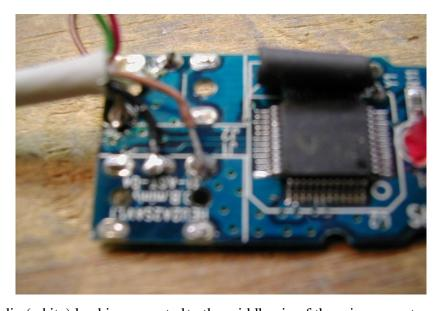
Note that the rxaudio (white) lead is connected to the middle pin of the mic connector at the top.
