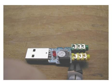
Once the connections are free on the outsides of each jack, rock them back and forth to cause the inner connections to break free as shown:
