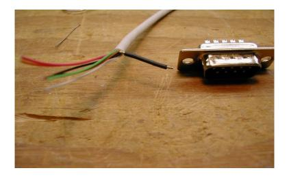
We can now attach the wires which connect directly to the connector pins. These would be ground, COR and PTT. The cable shield (ground) gets soldered to pin 5. The PTT (red) lead gets soldered to pin 7, and the COR lead (green) gets soldered to pin 4:
