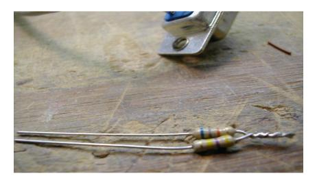
The center of the divider goes to the rxaudio (white) wire (Note: the picture shows the black wire which is wrong). The loose end of the 68K resistor gets soldered to pin 5 with some plastic tubing slipped over the bare wire. The loose end of the 470K is soldered to pin 3 of the D-sub connector:
