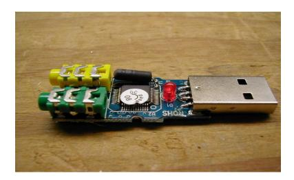
Peel the QC sticker off the chip and verify it is a CM108. If it isn't a CM108, it cannot be used. Then using a pair of precision cutters, remove the 3.5mm jacks by cutting the metal connections on the side of the jack as shown:
