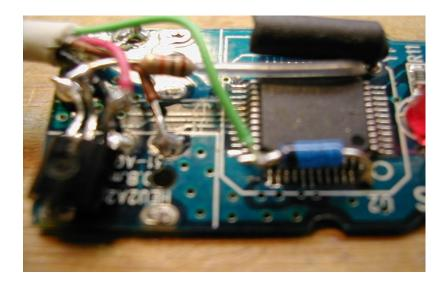
Finally, because of the way the parts are mounted, it would be a good idea to secure the diode and transistor with some glue. I used hot melt glue as it is removable. Silicone RTV should be avoided due to its acid content.
