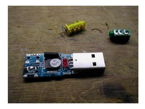
Do not be tempted to clean out the pins from the holes used by the jacks, The traces on the board lift very easily.
