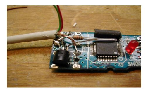
The free end of the 10K resistor attached to the middle pin (base) of the 2N4401. The transistor is mounted flat side down and the leftmost lead (emitter) is soldered to ground at the same point used by the cable shield. Note that the crystal was bent back down to its original orientation.
