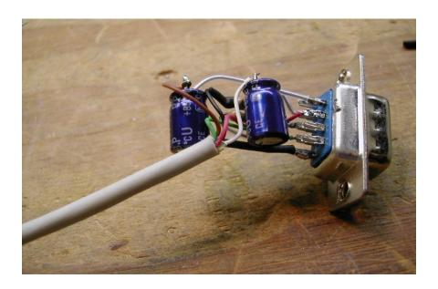
Once all of the parts are soldered in place, install the hood and position the parts and the wires so that they are not crimped by the connector hood:
