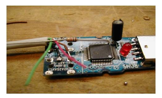
Next, we attach the 2N4401 transistor as shown:
