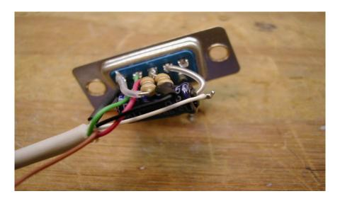
The auxiliary audio (brown) wire is the last connection to be made. It is connected through a 10 microfarad nonpolarized capacitor to pin 5 of the D-sub connector. Be sure to use plastic sleeving over the bare capacitor lead to avoid a short circuit:
