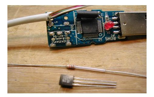
Now we connect some wires to points on the board. For the multiconductor cable I'm using, white is receive audio, black is transmit audio, brown is auxiliary audio, red is PTT, and green is COR. For now we will solder down the receive audio (white), transmit audio (black), and auxiliary audio (brown) wires as shown:
