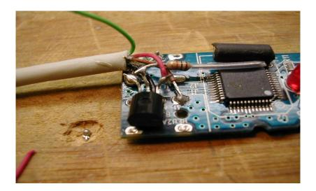
Now we prep the BAT43 diode similar to how we prepped the 10K resistor and solder the prepped end to pin 48 of the CM108, and the other end to the COR (green) wire. Note that the banded end (cathode) of the diode connects to the green wire:
